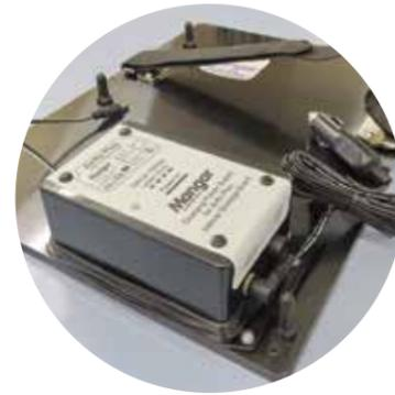
The stowage board secures the Airflo Plus in place and protects it when the vehicle is on the move. Using a stowage board also means ambulance crews can quickly locate the Airflo Plus in an emergency situation.
